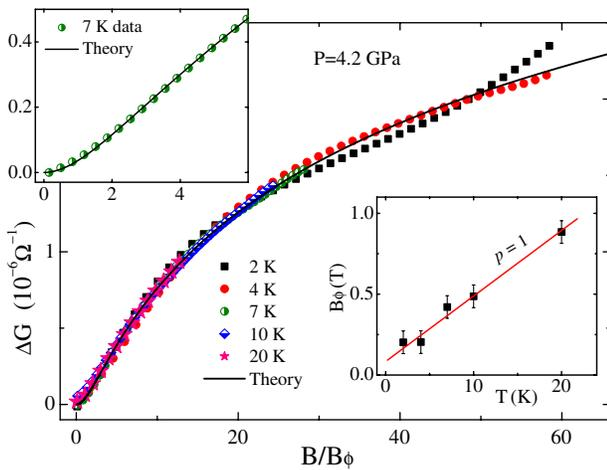
FIG. 3 (color online).  $\Delta G$  at different temperatures as a function of scaled field ( $B/B_\phi$ ) collapse onto a universal curve (the solid line), as described by Eq. (1) predicted by the 2DWL theory. Upper left inset: detailed comparison in low fields between the data measured at 7 K and theory. Lower right inset: the fitting parameter  $B_\phi$  vs temperature, showing a linear dependence corresponding to  $p = 1$ .
